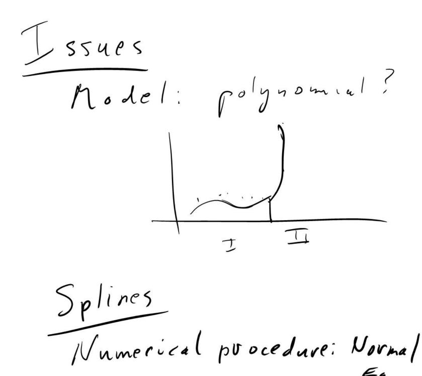
X: vary greatly  $f_{1}(x) = a_{0} + a_{1}(x-\mu) + a_{2}(x-\mu)^{2} + - + a_{1}(x-\mu)^{2}$ Je (x1 = bogolx) + . . + b, ge (x) Je (x): poly of dagree k  $\sum_{i=1}^{k} g_r(x_i) g_s(x_i) = 0 \quad r \notin s.$ orthogonal.
