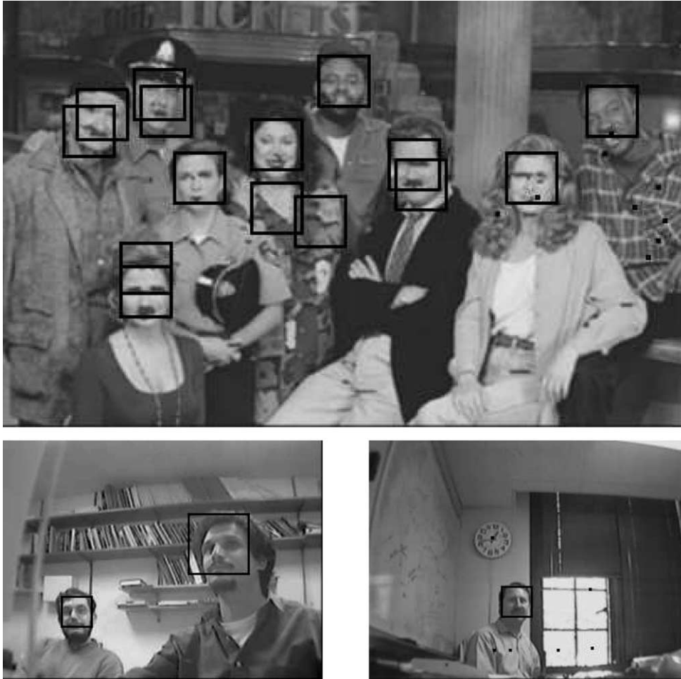
Fig. 10. Example of face detection and classification against non-face. The black dots denote all detections found in the image. The squares denote those detections that were classified as face.
