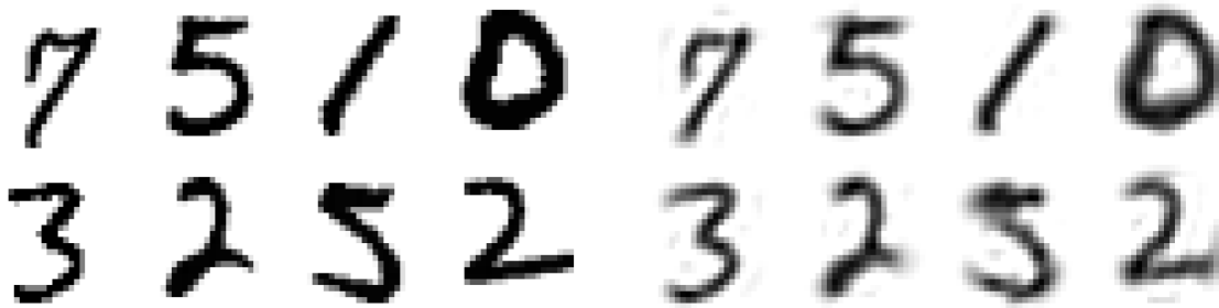
Figure 16: Left : Original MNIST handwritten digits. Right : MNIST handwritten digits projected onto the first fifty principal components.
