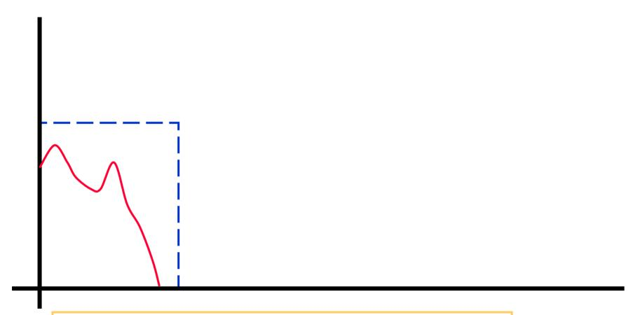
Crude quantization at extremely high rate + low-pass filter = 1-bit CD player ("Bitstream")
