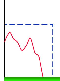
Crude quantization at extremely high rate + low-pass filter
