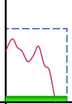
Crude quantization at extremely high rate + low-pass filter
